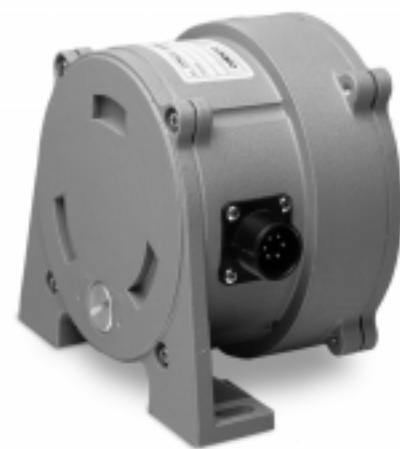
The model IT9420 is a rugged and simple device which provides a 4 to 20 mA current feedback signal for incline position. The heart of the IT9420 is a magnetically-damped pendulum coupled to a conductive plastic precision potentiometer. A highly linear relationship between inclination and a 4 to 20 mA output is maintained over the full range of the IT9420.
