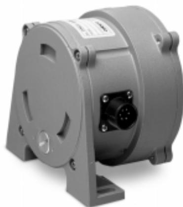
The model IT9101 is a rugged and simple device which provides a voltage diveder feedback signal for incline position. The heart of the IT9101 is a magnetically-damped pendulum coupled to a conductive plastic precision potentiometer. A highly linear relationship between inclination and the output signal is maintained over the full range of the IT9101.
